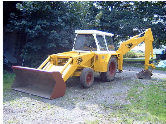
A "backhoe loader" A restored JCB 3C MkII, showing the conventional arrangement of front loader and backhoe
