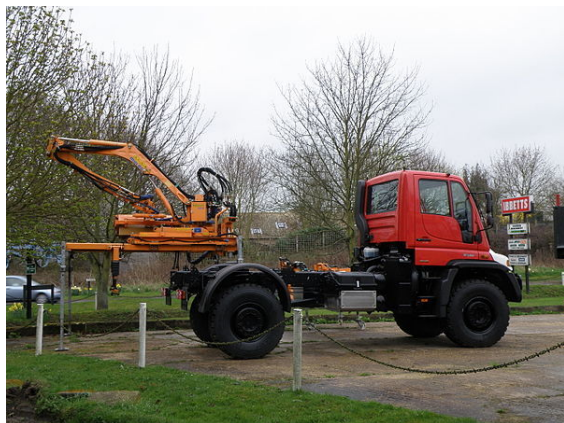
Unimog with a flail hedge and verge trimmer implement used in agroforestry
