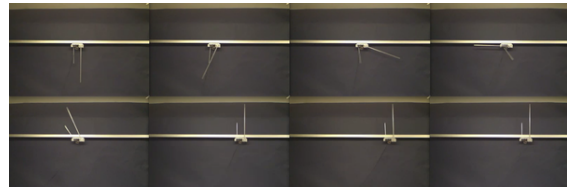
Smooth nonlinear trajectory planning with linear quadratic Gaussian feedback (LQR) control on a dual pendula system.
