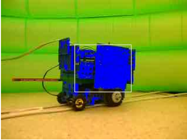
Figure 2: A camera image from the Rovio robot to which a blue blobify filter has been applied.
