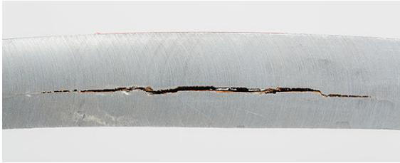
*Hydrogen Induced Cracks (HIC)*
